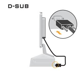
3. Insert the power cord into the monitor, then plug the monitor power cord and the computer cord into grounded electrical outlets.
